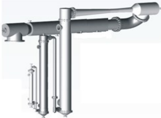
FOUR STAGE EJECTORS UNIT – OIL DEODORIZING
