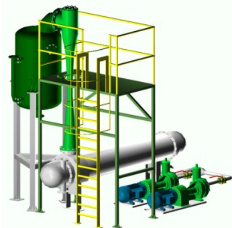
HYBRID VACUUM SYSTEM TO GENERATE COLD WATER EJECTOR AND WATER RING PUMP (WITH STAND-BY)
